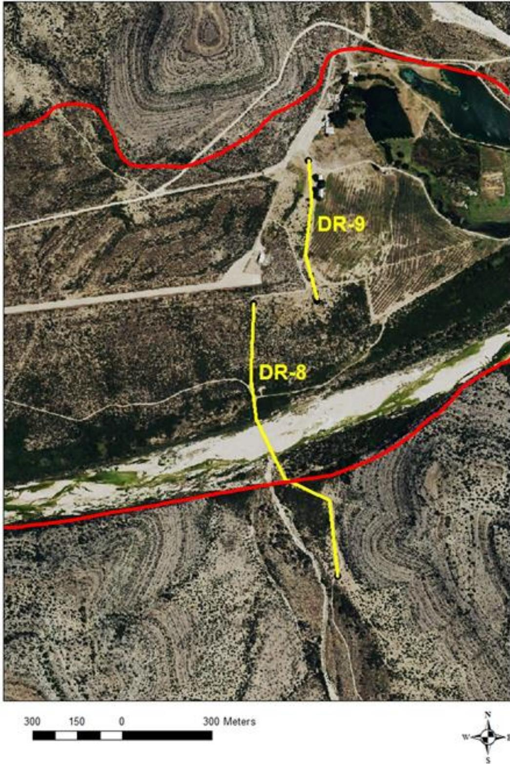
Figure 10. Close in view of the location of the electrical resistivity geophysical survey transect that crosses Independence Creek (denoted with yellow). The flood plain of Independence Creek is denoted in red.
