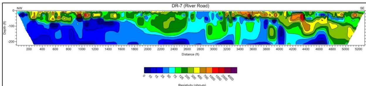
Figure 11. Electrical resistivity transect DR-7, located along River Road where it crosses Live Oak Creek. Resistivity is in ohm-m.
