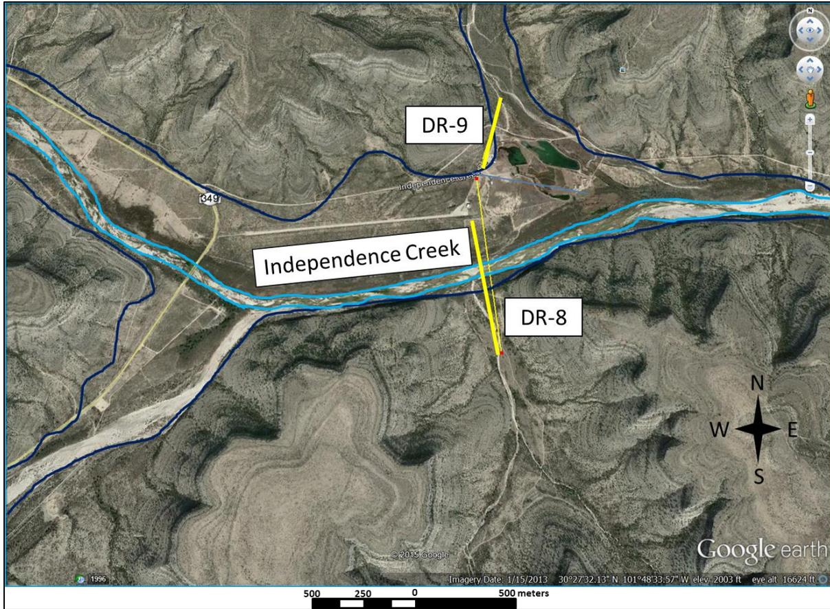
Figure 9. Location of the electrical resistivity geophysical survey transect that crosses Independence Creek (denoted with a yellow line). The main active channel of Independence Creek is denoted in light blue. The extents of the flood plains are interpreted as where limestone bedrock crops (dark blue line).
