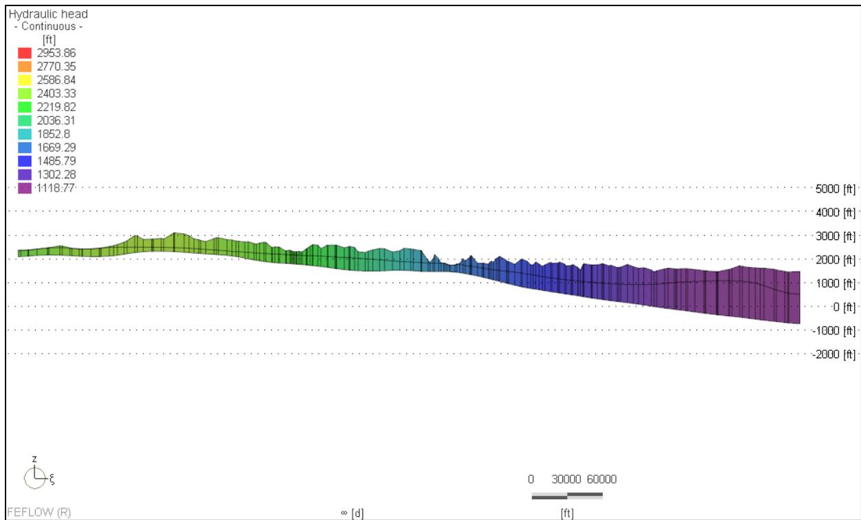
Figure 15. Model cross-section along two-dimensional Polyline #2 (shown in Figure 14). In the model domain, the Edwards-Trinity Aquifer thickens from <200 ft in the north to >2,000 ft in the south. Cross-section is colored according to the scale for hydraulic head.
