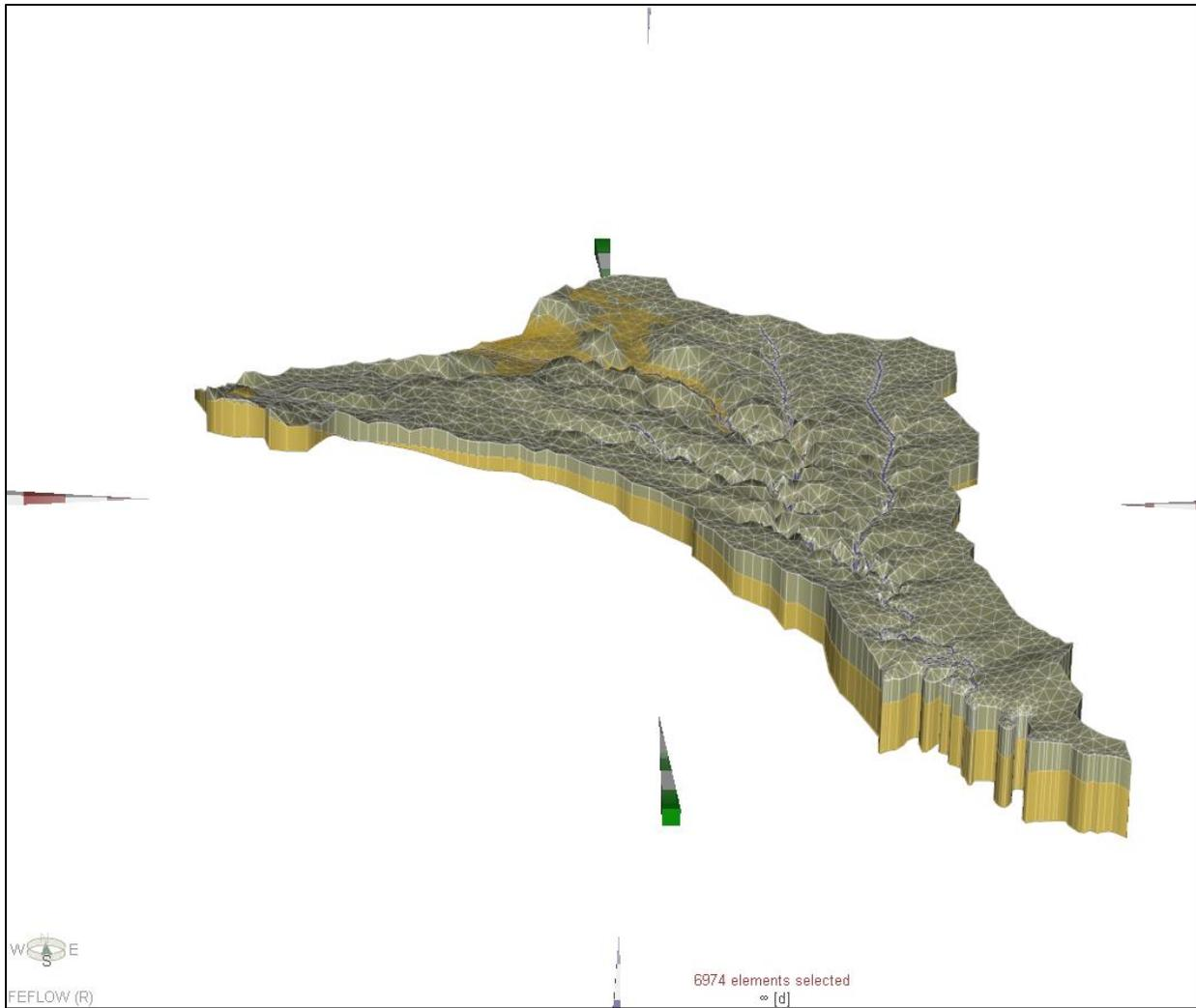
Figure 14. Oblique view of the model mesh looking from the south to the north. The current model consists of two layers, one each for the Edwards and Trinity rock units.
