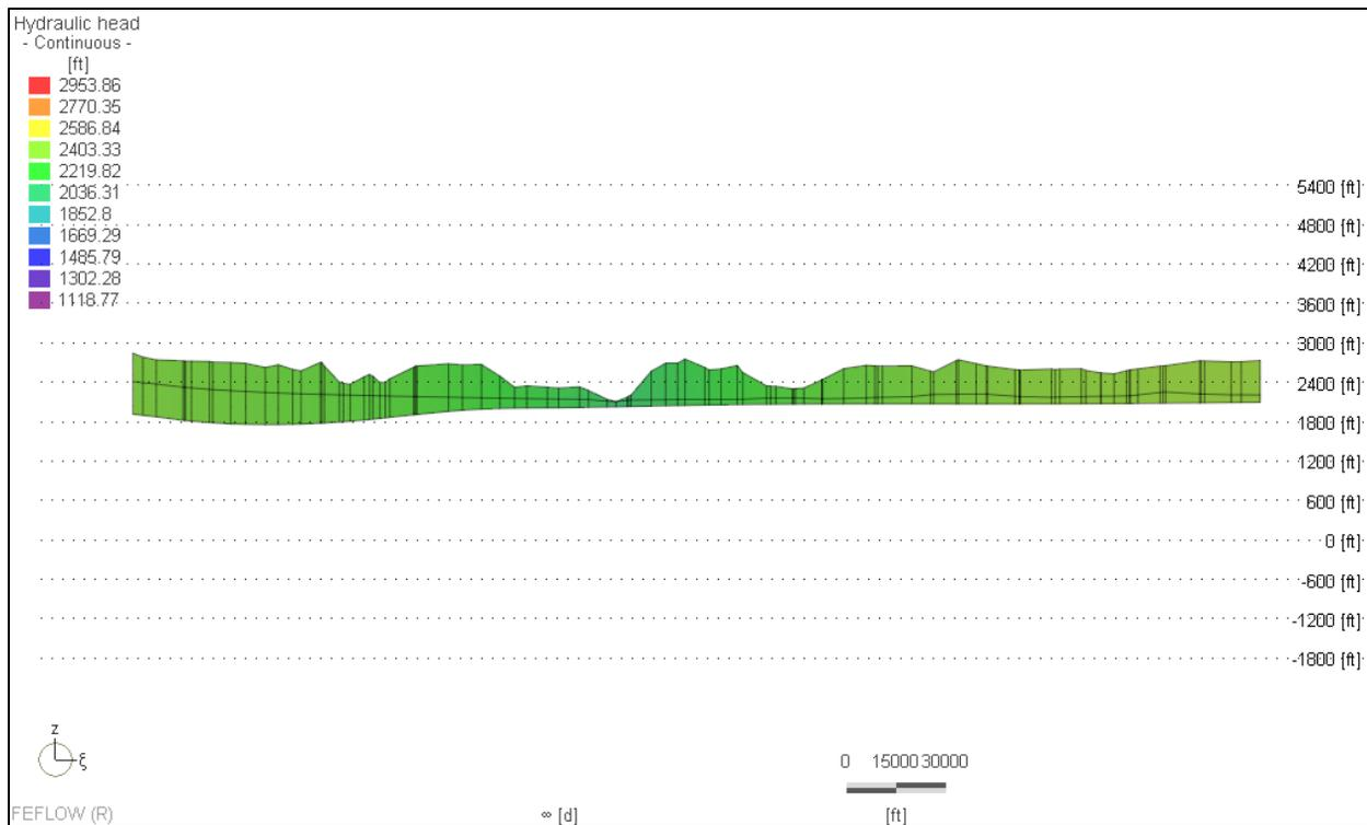
Figure 16. Model cross-section along two-dimensional Polyline #3 (shown in Figure 14). The Edwards-Trinity aquifer is incised by the Pecos River, with the Edwards sequence completely eroded in many sections of the Pecos River.
