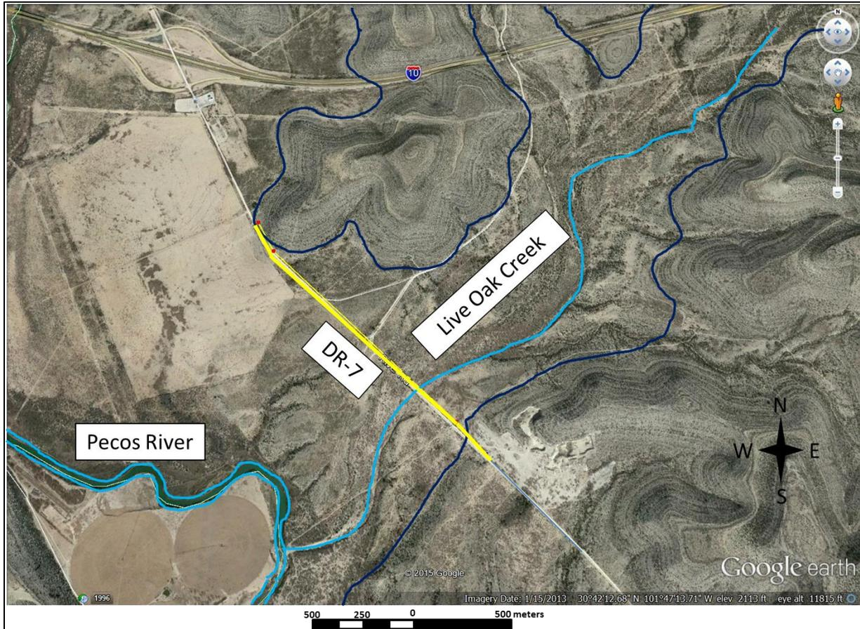
Figure 8. Location of the electrical resistivity geophysical survey transect that crosses Live Oak Creek (denoted with a yellow line and red boxes). The main active channels of Live Oak Creek and the Pecos River are denoted in light blue. The extents of the rivers' flood plains are interpreted to coincide with limestone bedrock outcrops (dark blue line).
