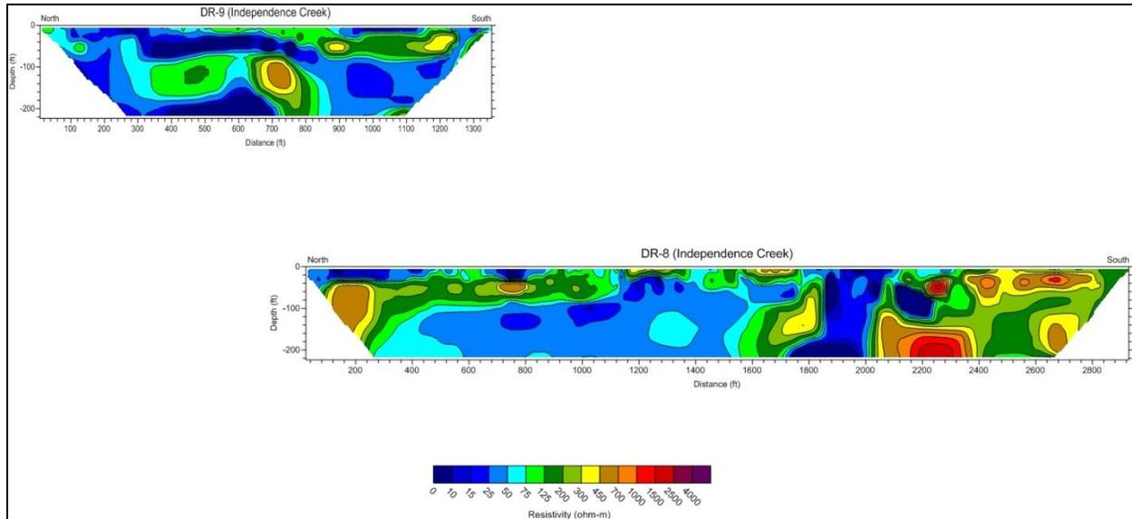
Figure 12. Electrical resistivity transects DR-8 and DR-9, located at the Oasis Ranch on Independence Creek and approximately two miles west of the confluence of Independence Creek within the Pecos River. Resistivity is in ohm-m.
